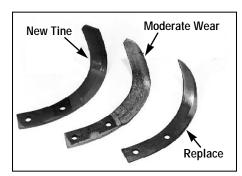
Figure 5-5: Checking tines for wear.
